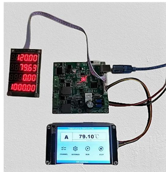
**OETTC-200 Heater Temperature Controller (OEM)**
